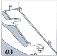
3. Place the first board against the wall. Provide a space of 8mm between the board and the left wall with the help of wedges or spacers
