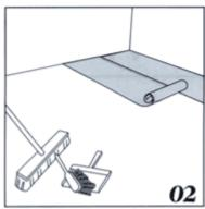
1. Check to see if doors open easily taking into account 2. After having cleaned the support floor, first lay the underlay strips side by-side (they can also be stapled into place).
