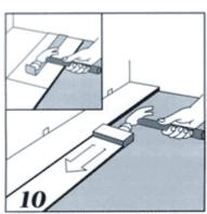
10. Assemble the short sides with the help of a tapping block stops at about 5 mm from the short side of the previous and a hammer Place the block on the floor against the far right end of the board and tap lightly until the far left end of the board and the far right end of the previous board tit perfectly together. Final installation of the last board of the row will be done with the help of a last board jemmy or a tapping bar as illustrated.
