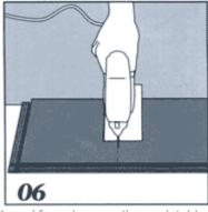
6. Place the board face down on the work table and saw with the help of a jigsaw. Use a fine blade if you use a handsaw, and in that case saw the board face up.
