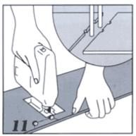
transfer the measurements and add 10 mm. After having cut the board according to the contours, put the cut piece again in place.
