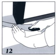
11. For plumbing pipes: measure the position of the pipes, 12. Door frames: cut the door frames with a saw while resting on one of the floorboards, so the floorboard can fit under it.
