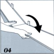
4. Place the second board against the first one at an angle and lay it flat on the floor. Press the second board firmly against the first Complete the first row in this manner.
