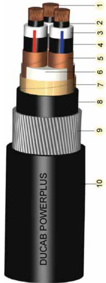
3.6/6 (7.2)kV Three Core Copper Conductors XLPE Insulated to IEC 60502-2 Steel Wire Armoured
