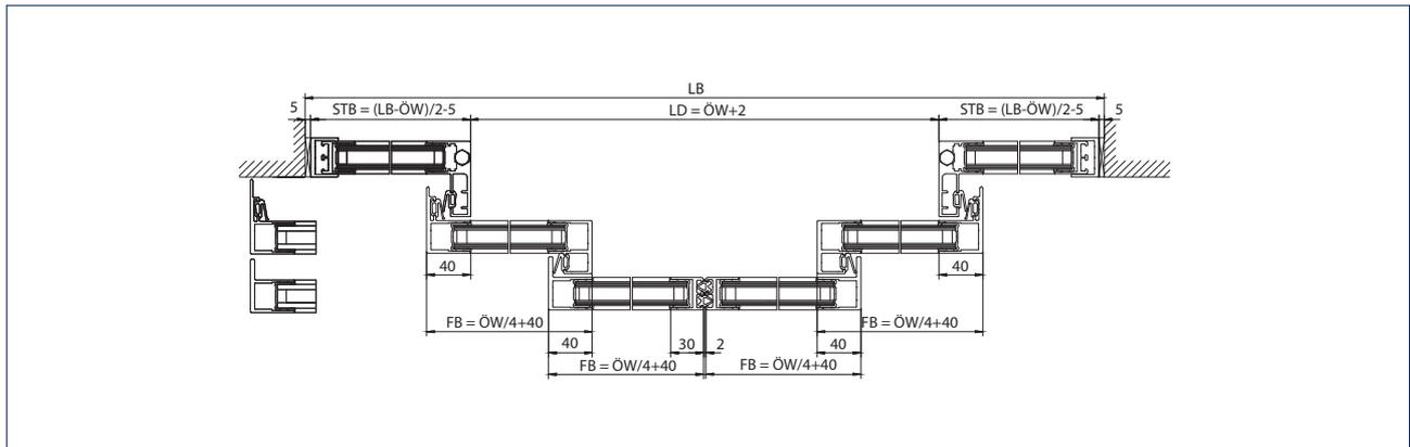
Installation: Wall mounting with longer drive and carrier between the walls
