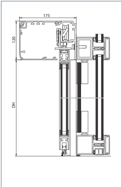
Installation: To post-rail structure with safety leaf
