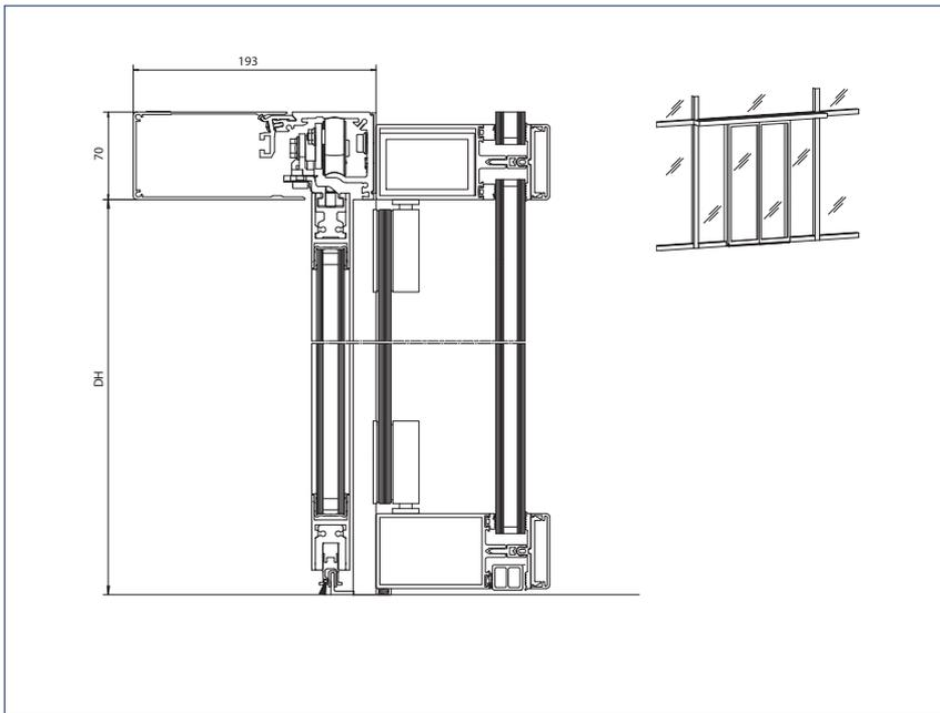
Installation: To post-rail structure with safety leaf
