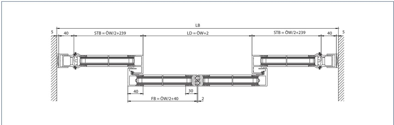
Installation: Cantilevered installation
