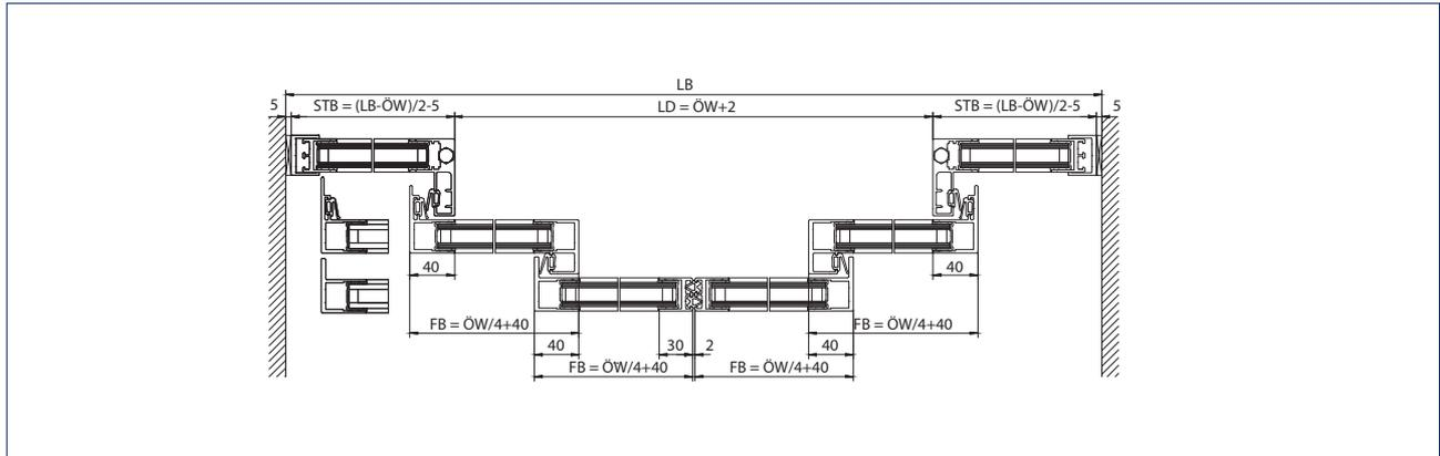
Installation: Cantilevered installation
