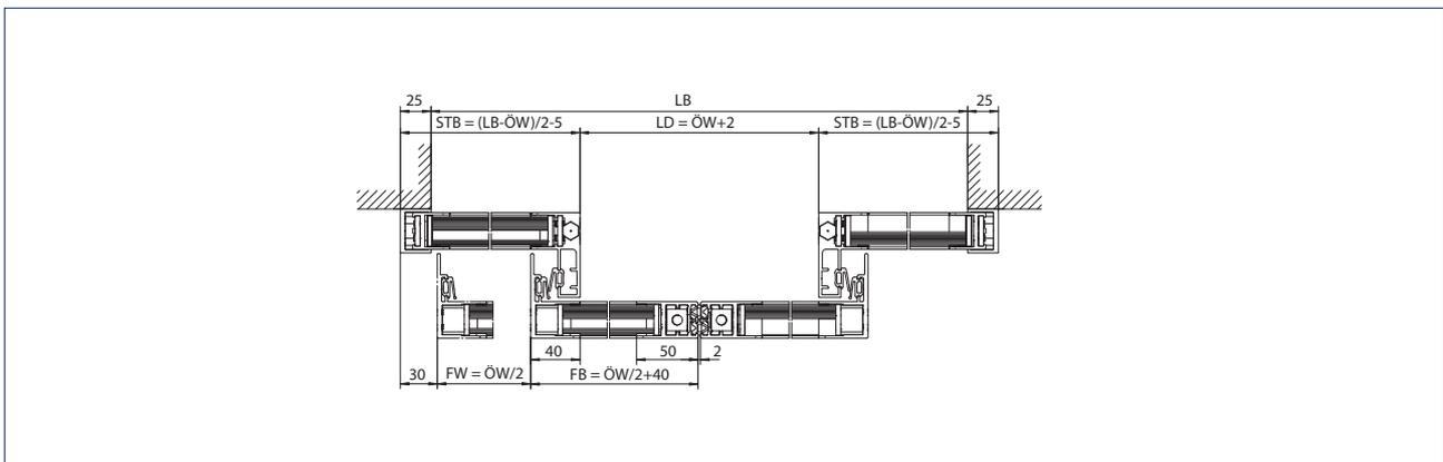
Installation: Wall mounting with side parts
