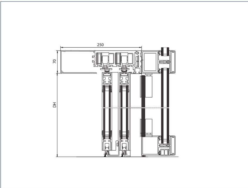
Installation: To post-rail structure with safety leaf
