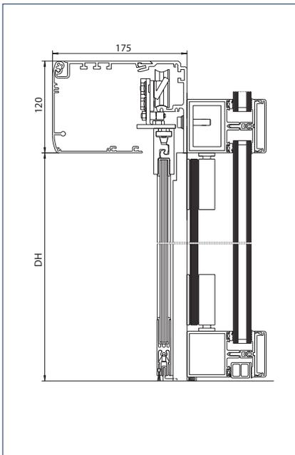
Installation: To post-rail structure with safety leaf
