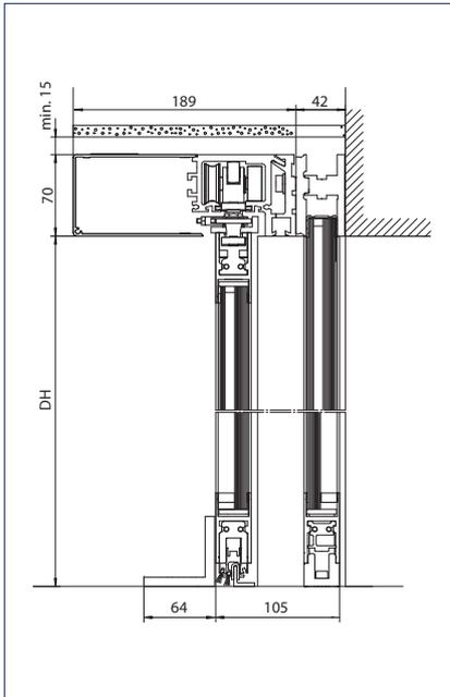
Floor guide: Pointwise with reinforced supporting bracket
