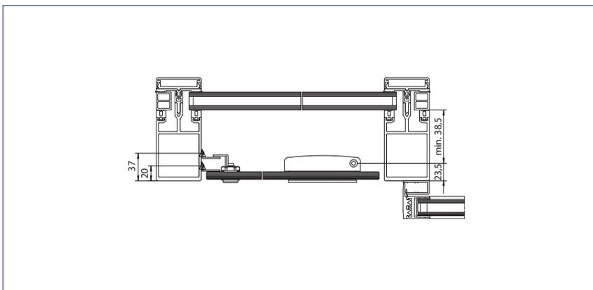
Installation: To post-rail structure with safety leaf
