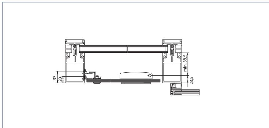
Installation: To post-rail structure with safety leaf
