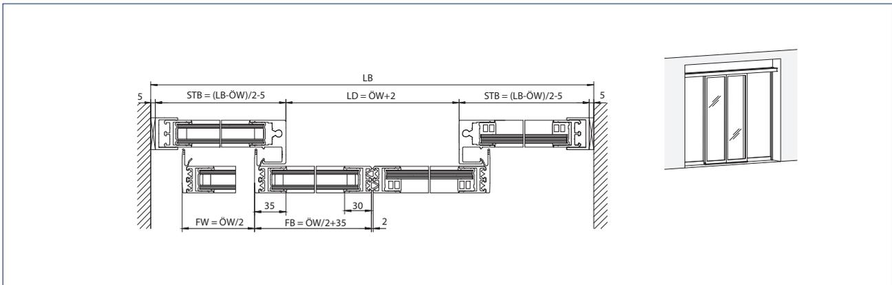
Installation: Cantilevered installation
