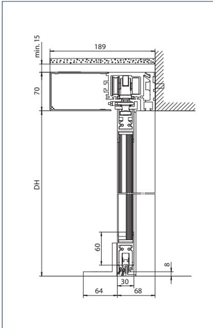
Floor guide: Pointwise with reinforced supporting bracket
