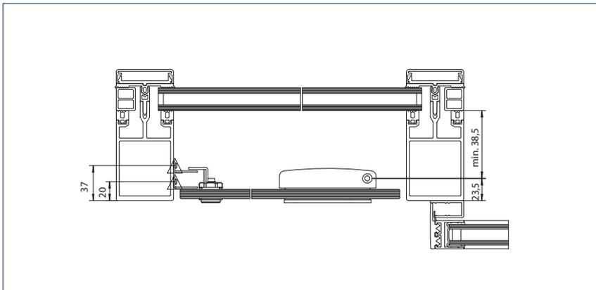
Installation: To post-rail structure with safety leaf
