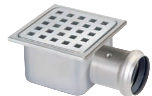
AQD-413-LOW-BS Shower Drain with Trap Horizontal Outlet Dia. 40 mm Capacity - 35 l/m 105 x 105 mm Low Height Brushed Stainless Steel
