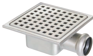
AQD-419-LOW-BS Floor Drain with Trap Horizontal Outlet Dia. 40 mm Capacity - 35 l/m 150 x 150 mm Low Height Brushed Stainless Steel
