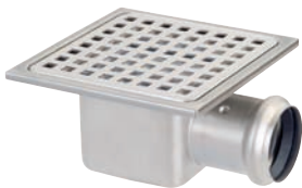
AQD-419-BS Floor Drain with Trap Horizontal Outlet Dia. 50 mm Capacity - 35 l/m 150 x 150 mm Brushed Stainless Steel
