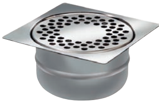
AQD-414-BS Floor Drain with Trap Bottom Outlet Dia. 50 mm Capacity - 18 l/m 150 x 150 mm Brushed Stainless Steel
