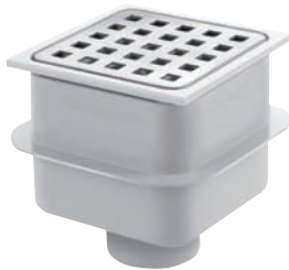
AQR-614-ABS-BS ABS Drain with Brushed Stainless Steel Grating Vertical Outlet Dia. 50 mm Capacity - 35 l/m 105 x 105 mm
