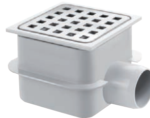
AQR-615-ABS-BS ABS Drain with Brushed Stainless Steel 304 Grating with Anti-odour 50 mm Water Seal with Removable Trap Horizontal Outlet Dia. 50 mm Capacity - 35 l/m 105 x 105 mm
