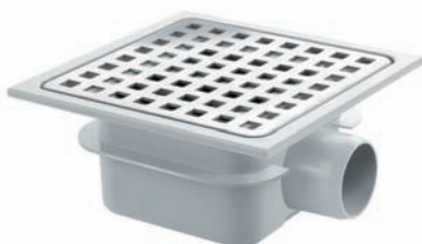
AQR-617-ABS-BS ABS Drain with Brushed Stainless Steel 304 Grating with Anti-odour 35 mm Water Seal with Removable Trap Horizontal Outlet Dia. 40 mm Capacity - 35 l/m 150 x 150 mm
