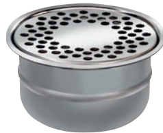
AQD-414-ROUND-BS Floor Drain with Trap with Anti-odour 50 mm Water Seal Bottom Outlet Dia. 50 mm Capacity - 18 l/m Dia. 150 mm Brushed Stainless Steel
