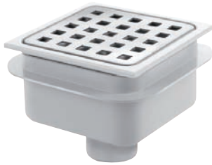
AQR-612-ABS-BS ABS Drain with Brushed Stainless Steel 304 Grating with Anti-odour 35 mm Water Seal with Removable Trap Vertical Outlet Dia. 40 mm Capacity - 35 l/m 105 x 105 mm
