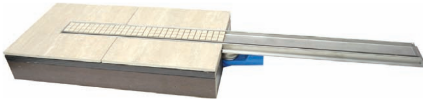
Premium Line Shower Channel with Plastic 90° Bend (Outlet Horizontal) and Removable Plastic Trap (RSA) Complete with Reversible Tray for Tile Installation Capacity: 35 l/m
