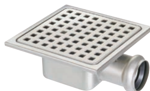
AQD-419-LOW-BS Floor Drain with Trap (Low Height) with Anti-odour 35 mm Water Seal with Removable Trap Horizontal Outlet Dia. 40 mm Capacity - 35 l/m 150 x 150 mm Brushed Stainless Steel
