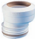
MUL-MK02 OFFSET Used when the Soil Pipe and WC Pan Spigot are misaligned 18 mm Offset with Pipe Size 99 mm - 105 mm (I.D)
