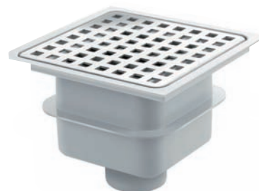
AQR-618-ABS-BS ABS Drain with Brushed Stainless Steel 304 Grating with Anti-odour 35 mm Water Seal with Removable Trap Vertical Outlet Dia. 50 mm Capacity - 35 l/m 150 x 150 mm
