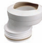
MUL-MK04 OFFSET Used when the Soil Pipe and WC Pan Spigot are misaligned 40 mm Offset with Pipe Size 99 mm - 105 mm (I.D)
