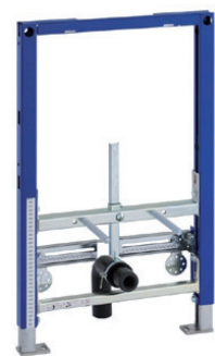
GEB-111-524-00-1 Duofix Element for Bidet for Installation in Dry Wall or Pre-Wall Construction, Covered with Panel (Gypsum or Wood), for a Floor Construction of 0-200 mm Installation Height Approx. 820 mm
