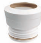
MUL-MKS1 STRAIGHT Used when the Soil Pipe and WC Pan Spigot are Aligned 108 - 114 mm (O.D) and soil pipe 99 - 105 mm (I.D)
