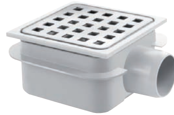
AQR-613-ABS-BS ABS Drain with Brushed Stainless Steel 304 Grating with Anti-odour 35 mm Water Seal with Removable Trap Horizontal Outlet Dia. 40 mm Capacity - 35 l/m 105 x 105 mm
