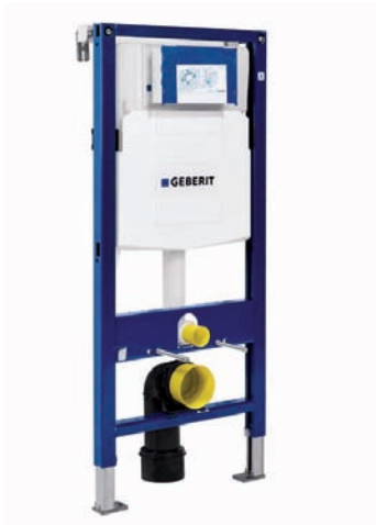
GEB-111-300-00-5 UP320 Duofix Concealed Cistern for Wall Hung WC For Installation in Dry Wall Construction Installation Height Approx. 1120 mm Thickness 120 mm
