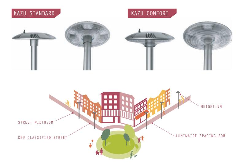
The Kazu offers a very competitive solution compared to luminaires fitted with mercury and high-pressure sodium lamps for lighting this typical CE3 classified street (according to CIE 115) with a return on investment in less than 4 years and energy savings of up to 83%.
