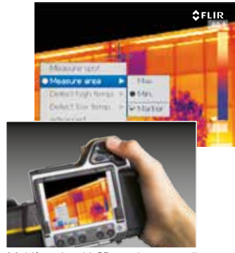
Multifunctional LCD touch screen allows quick and easy camera software menu handling.
