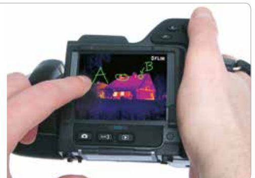
Thermal image of the same building, now using the MSX-setting. Note that more details are visible, making it easy to locate ventilation grids and see brick structure. The MSX feature gives depth to your thermal image.
