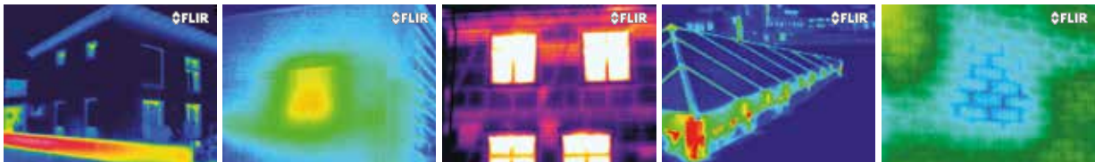
Thermal image shows insulation quality of a low energy house.
