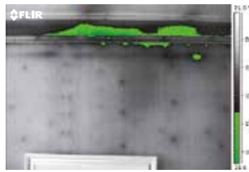
The insulation alarm shows where the areas below or above a set temperature are by making them appear in a different color.
