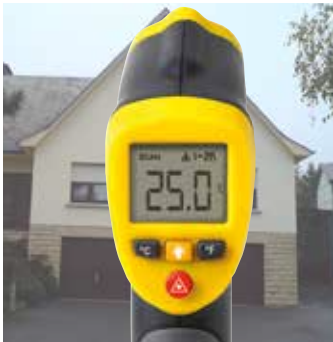
IR thermometer, temperature measurement in one spot
