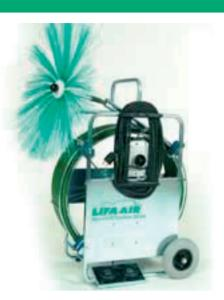
Lifa Special Cleaner 20 is an electrically powered ventilation duct cleaning machine with a rotation speed of 550 r/minute. It is designed to clean the inside surfaces of small ducts in the Ø 100-600 mm range, although 400-600 mm ducts can only be vertical flues.
