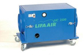
HepaClean 2500 is intended for cleaning dry air containing asbestos, mould, construction, quartz, powder or wood dust. When the machine is equipped with an active carbon filter, gaseous compounds can be removed. The machine can also be used to create negative pressure in rooms and compartments.
