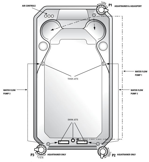
The pump 2 and pump 3 (P2 & P3) DIVERTER valves provide variable water flow adjustment between the two upper swim jets (providing variable swim resistance), and the two thigh jets on either side of the swim spa (providing variable resistance for water-aerobic excercises or hydrotherapy needs).
