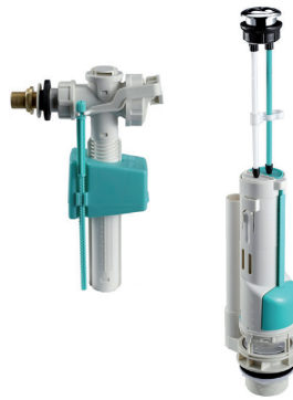
Side Inlet Mechanism Dual Flush - 3-6 Litres Adjustable Float - Variation 100 mm Pressure Ranges 0.3 - 10 bar Connections - 3/8" in brass to convert to 1/2" Plastic AQE-B9352-ESG1 must be purchased Universal Installation for most European WC Cisterns Code: AQE-T001-SI
