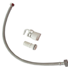
Mechanism Converter Kit Converts AQS-T001-SI Side Inlet Mechanism to be Used in a Back Inlet Cistern that has a Cut Out Includes Thread Converter, Clip and Flexible Hose Connects to 3/8" Male Connection Code: AQE-B9352-ESG1
