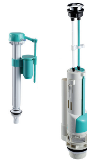
Bottom Inlet Mechanism Dual Flush - 3-6 Litres Adjustable Float - Variation 75 mm Pressure Ranges 0.3 - 10 bar Connections - 1/2" in plastic Available With or Without Refill Function Code: AQE-T001-BI
