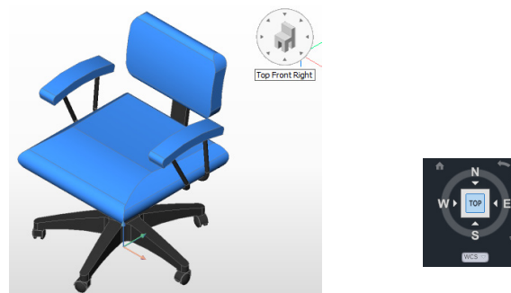
Left: LookFrom control in BricsCAD; right: equivalent ViewCube control in AutoCAD
