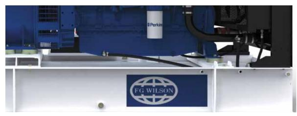
The fuel tank design incorporates a reinforced sloped top plate for liquid run off, acting as a catchment area for all potential liquid spills and leaks. A sloped bottom plate and notched drain plug allows for efficient, controlled drainage of the fuel tank. The fuel tank is designed for 8 hours running at full load in prime applications.
