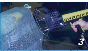
Shrink the material with a heat gun until it is stretched tightly around the entire product.
