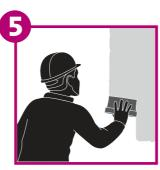
Apply 2nd coat in opposite direction to first coat (horizontal or vertical) in uniform thickness of between 0.5mm to 2mm. As plaster progressively sets, trowel to a smooth finish removing scratches and unwanted material by putty knife, trowel or finishing tools.
