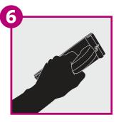
Prior to application of primer, allow to dry completely. Gently level the minor undulations on the wall with fine sand paper of 180 - 200 grit to attain a smooth finish.
