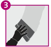
After complete mixing of Gyproc GypFine - Board Skim, start applying first coat onto plasterboard wall or ceiling, in uniform thickness of between 0.5mm to 2mm in any one direction (horizontal or vertical) by using a clean putty knife, trowel or any finishing tool.
