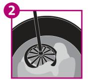
Proceed with mixing, using a hand mixer or machine mixer of 200rpm to make a uniform paste. Continue the mixing to form a homogeneous mix. Gyproc GypFine - Board Skim has an approximate working time of 110 minutes. Do not mix more than can be used as per the product recommendations.
