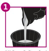
Add Gyproc GypFine - Board Skim to clean water in the ratio of approximately 10kg of powder to 7litres of water. After adding powder to water, wait 2 - 3 minutes before mixing.
