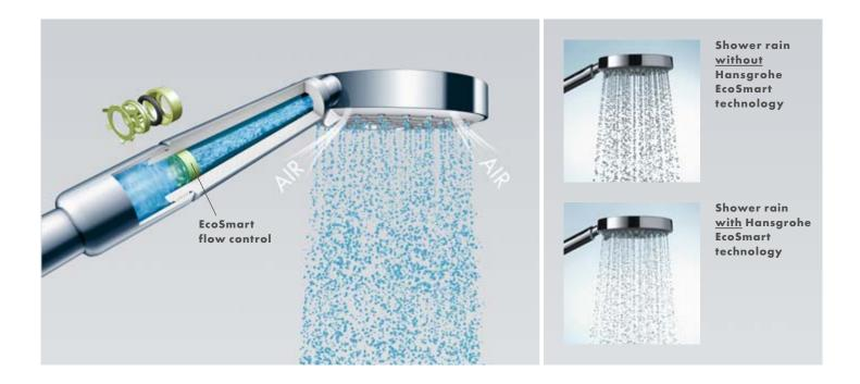
**EcoSmart technology.** How do you transform a little water into a whole lot of water? Simply by using Hansgrohe's EcoSmart technology. Sophisticated flow limitation, special spray jets and the mixing of water with air reduce water consumption down to either 6 or 9 l/min – while offering lots of shower comfort. It also saves energy, since less water needs to be heated. In this way, your daily contribution to climate protection begins under the shower.
