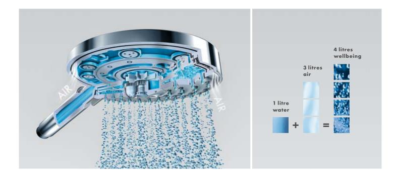
**AirPower Technology.** To use water more effectively, we like mixing it up with lots of air. Air is drawn in through the entire spray disc and mixed together with the inflowing water. About 3 litres of air are used for every litre of water! The result: the drops become more voluminous, lighter and softer. Water consumption remains constant while the pleasure increases – high efficiency, plenty of Shower Fun.
