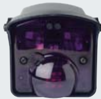
Comfort radar / presence detector Radar movement and presence detection with infrared detection. Fast and targeted automatic door opening. Reliable advance protection. Up to max. 6 m height. In areas with high levels of humidity and in outside areas, only the radar function is available. Housing: protection category IP 65.
