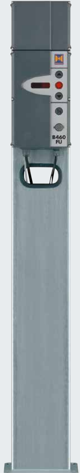
Optional: Key switch post ST1 1 For installing a maximum of 2 controls with additional housing. Colour: White aluminium, RAL 9006 Dimensions: 200 × 60 mm, height 1660 mm
