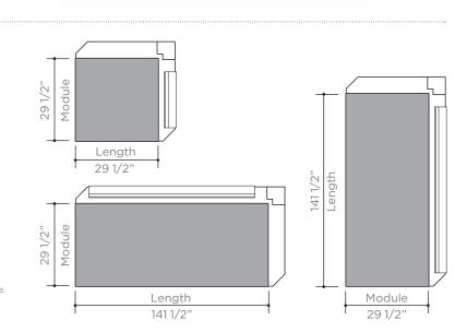
\*Various horizontal and vertical reveal options available. Contact CENTRIA for details. \*\*Panel depths are available from 1 3/8" to 4".
