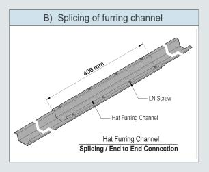
These details represent some of the most common designs situations relevant to the Knauf KC A001 ceiling systems.
