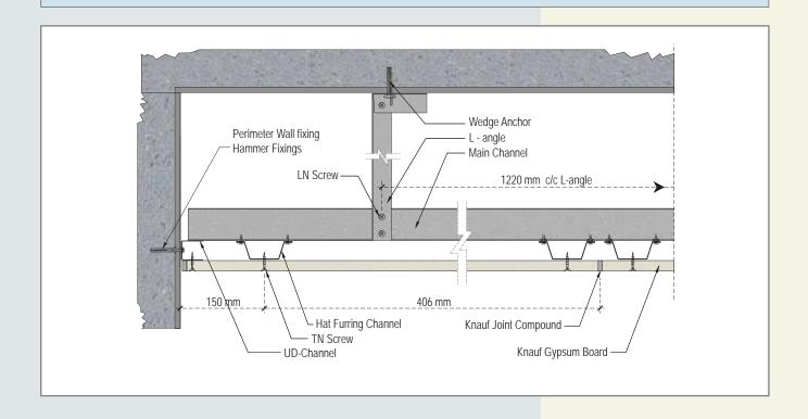
These details represent some of the most common designs situations relevant to the Knauf KC A001 ceiling systems.
