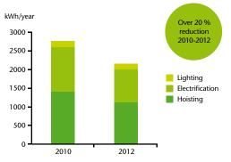
The basis for the calculation is an elevator speed of 1.6 m/s, a load of 1000 kg, 200,000 starts/year, a travel height of 45 m and 15 floors
