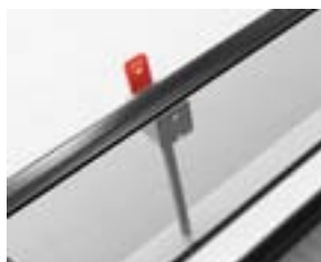
Additional emergency stop button (EN115-1:2008+A1:2010 requirement)
