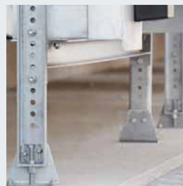
Adjustable pedestal feet Height-adjustable supports allow adjustment of the pedestal level, even subsequently (e.g. after lowering of the building). Pedestal feet are always galvanised.
