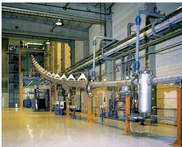
Fig. 2 Continuous Vulcanization (CV) Line
