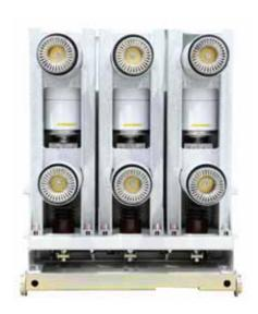
Which condenses on the surrounding metal shield. At current zero the arc extinguishes and vapor production ceases. The metal vapor plasma is very rapidly dispersed, cooled, recombined, and deionized, and the metal vapor products are quickly condensed so that the contacts withstand the transient recovery voltage.
