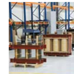
Special assembly benches for perfectly aligning the cores to the right positioning references.
