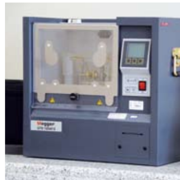
Transformer Oil B.D.V Tester
