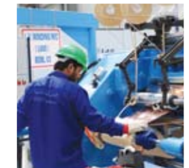
4- Low Voltage Winding
