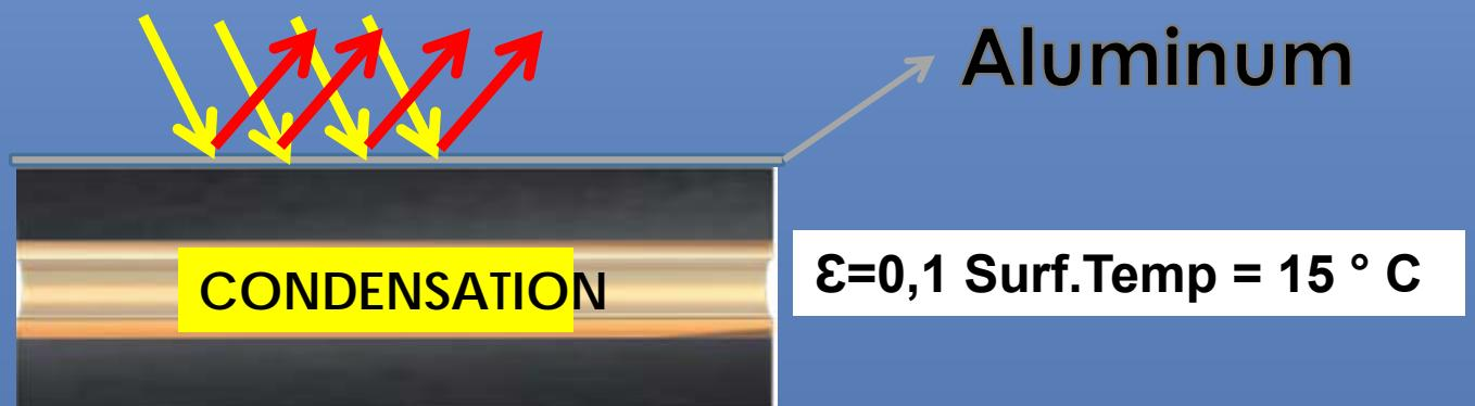
Aluminium foil      low emissivity absorption and a lower surface temperature.
