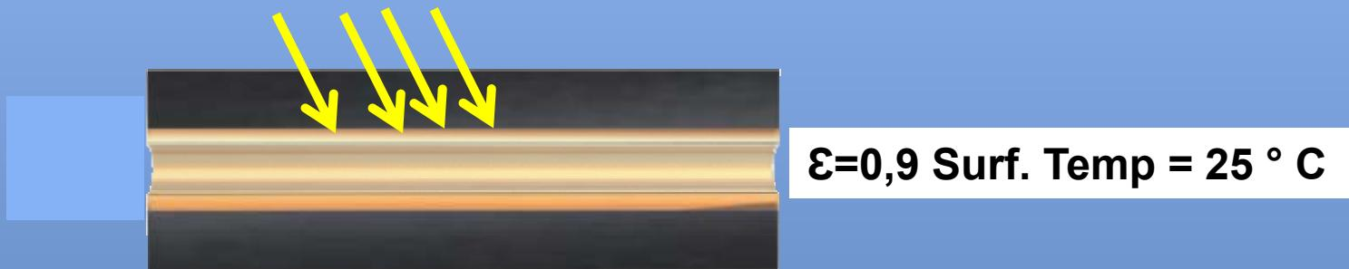
BLACK      High emissivity absorption and a higher surface temperature.
