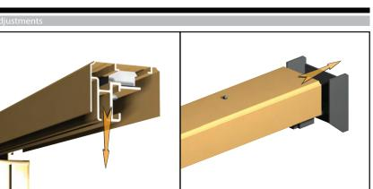
The upper track can be regulated for up to 8mm.
