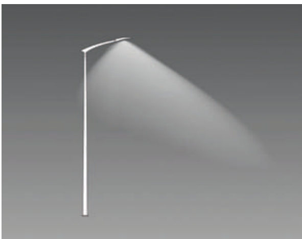
Light distribution without Back Light Control
