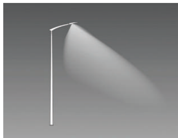
Light distribution with Back Light Control
