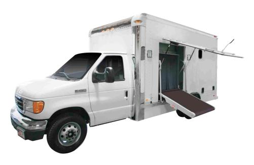
With a tunnel opening of 1010 x 1010 mm (39.8" x 39.8"), the XIS-Van offers a large tunnel capable of screening mail, baggage and freight for explosives and contraband. The XIS-Van offers optional 4 Wheel Drive and is built for use on both urban and rugged terrain.
